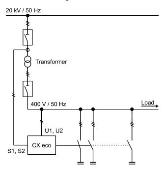
The reactive power caused by the transformer is measured by a medium-voltage current measurement and compensated by the connected compensation system.
