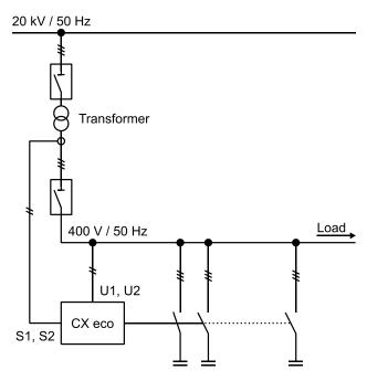
If there are no static stages available to compensate an upstream transformer, this can be done by the control of the CX eco.
