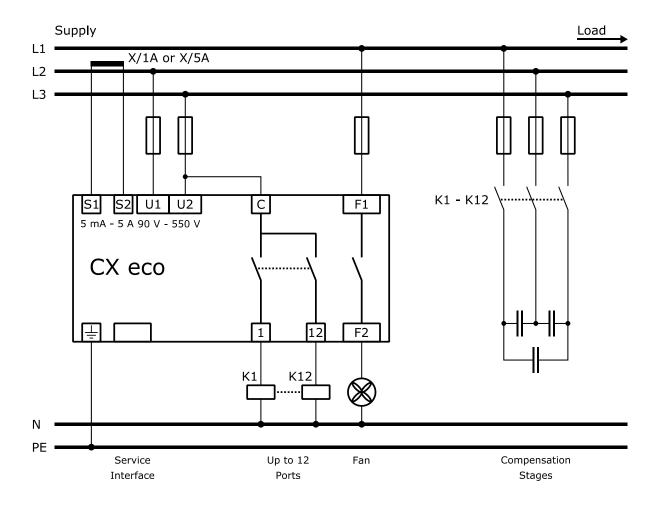
**NOTE:** The CX eco is designed to control **capacitive or inductive** stages. Operating both stage types simultaneously is not possible.
